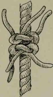
FIG. 118.—Shroud knot (making).
